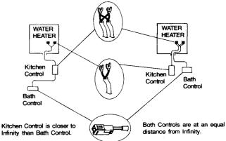
Cables are simply piggy-backed at the Infinity or the Kitchen Control. Polarity is not important when connecting cables.
