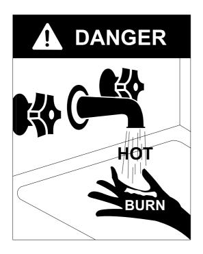
Water temperatures over  $50^{\circ}\text{C}$  can cause severe burns instantly or death from scalds.
