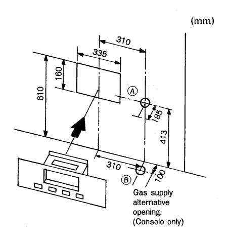
When using supply alternative (B) the pipe is fed from underneath, through the opening in the base.
