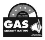
Comparative Energy Consumption tested to The Australian Gas Association requirements of Australian Gas Code AG 103. An energy rating of 5 stars refers to an efficiency of approximately 80%, that is, 80% of gas consumed is converted to useful heat.
